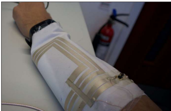
A silver/carbon component makes this ‘smart bandage’ possible.
